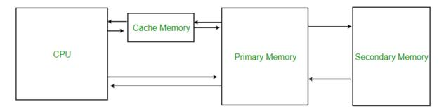
When the processor needs to read or write a location in main memory, it first checks for a corresponding entry in the cache.
