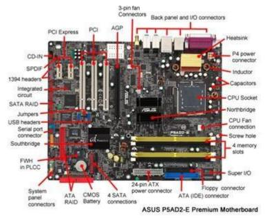
It is a printed circuit board that is the foundation of a computer, located at the bottom of the computer case. It allocates power to the CPU, RAM, and all other computer hardware components. Most importantly, the motherboard allows hardware components to communicate with one another.
