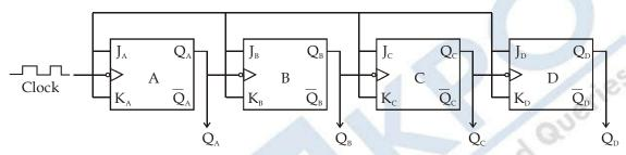
A binary ripple counter is constructed using clocked JK-flip flops.
