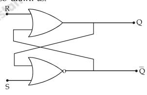
Q is O/P of the flip-flop. Q is the complement of the O/P. Thus a high on S (Keeping R = O) i/p will make. Q =). Q is one of this i/p's to the upper NOR gate. As both i/p (R & Q) of the upper NOR gate an now low, its output Q until be high. Thus, the flip-flop stores binary bit 1 when 8 is made high. Even of the set i/p S is removed, the O/P Q will remain 1 because Q is one of the i/ps of the lower NOR gate.  $111^{ly}$ , when reset input R is mad, high keeping S = 0, Q will become low.
